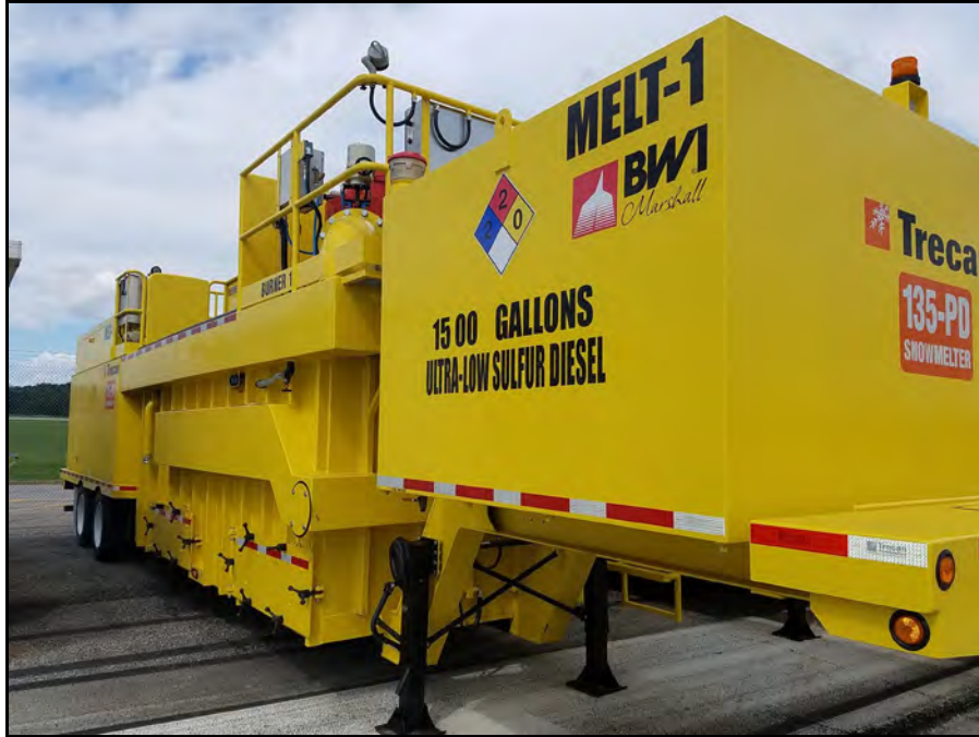
Mobile AST (MELT-1) affixed to Snow Melter Unit in the Long Term B Parking Lot
