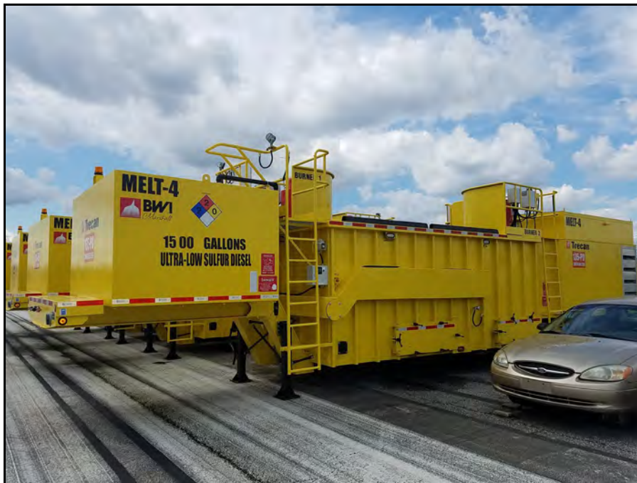
Mobile AST (MELT-4) affixed to Snow Melter Unit in the Long Term B Parking Lot
