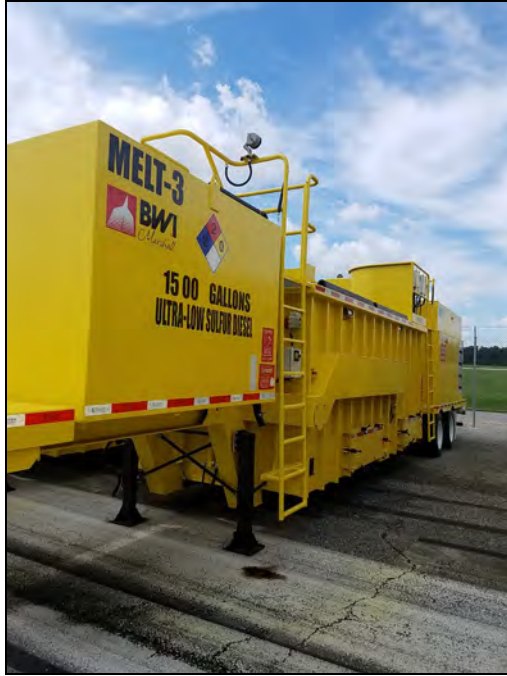
Mobile AST (MELT-3) affixed to Snow Melter Unit in the Long Term B Parking Lot
