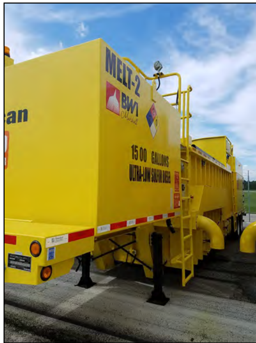
Mobile AST (MELT-2) affixed to Snow Melter Unit in the Long Term B Parking Lot
