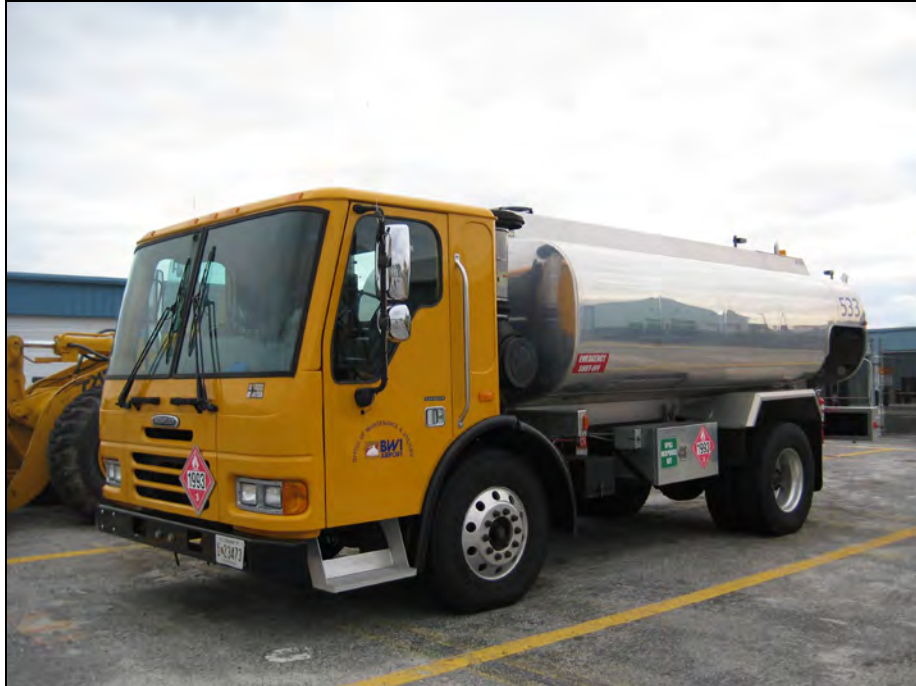
2,700-Gallon Mobile Refueler (Tank Truck 533) Normally Parked At Field Maintenance Facility between Building 115 and Building 158
