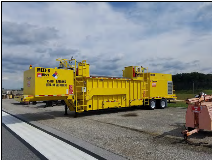
Mobile AST (MELT-8) affixed to Snow Melter Unit in the Long Term B Parking Lot
