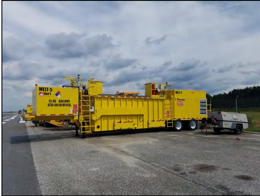
Mobile AST (MELT-5) affixed to Snow Melter Unit in the Long Term B Parking Lot
